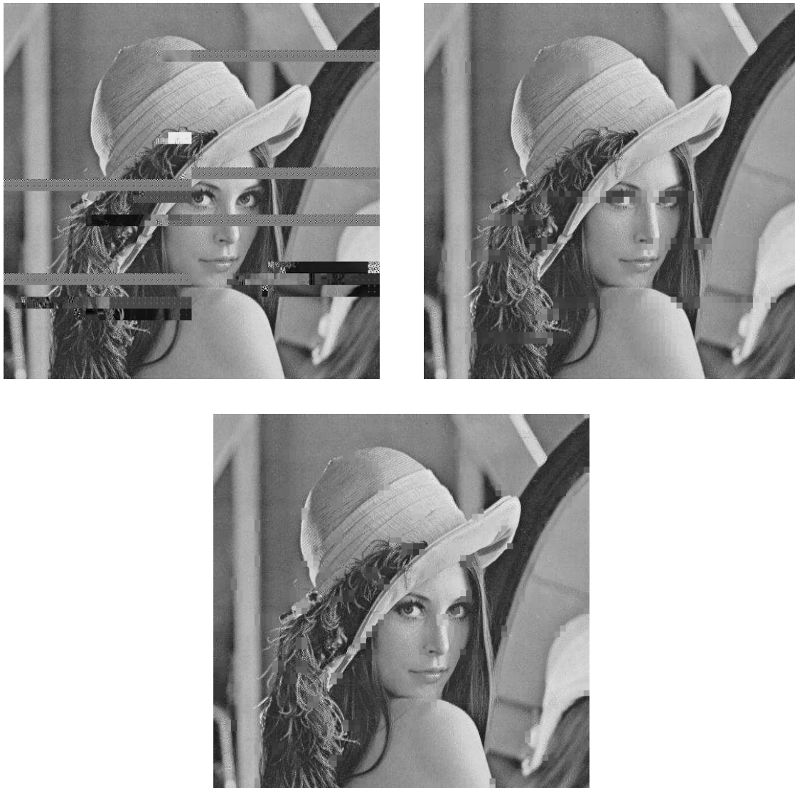
Figure 6 : Three decoded images which have been transmitted using (a) JFIF (b) Layered and (c) DSJ formats. Each image has suffered 10% cell loss.
